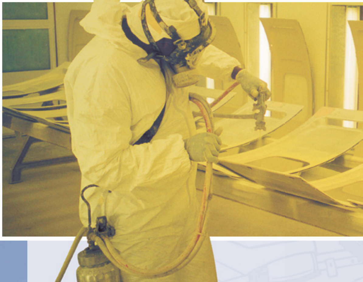
Spray application of the polyurethane coating
